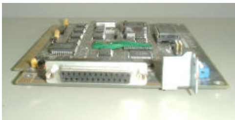
Figure 2. Communication Server Drive Card
