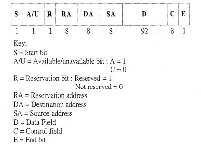
Fig. 3 Packet format for the slotted ring network with reservation mechanism
