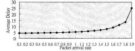
Fig. 2 Average Packet Delay for Slotted Ring Network
